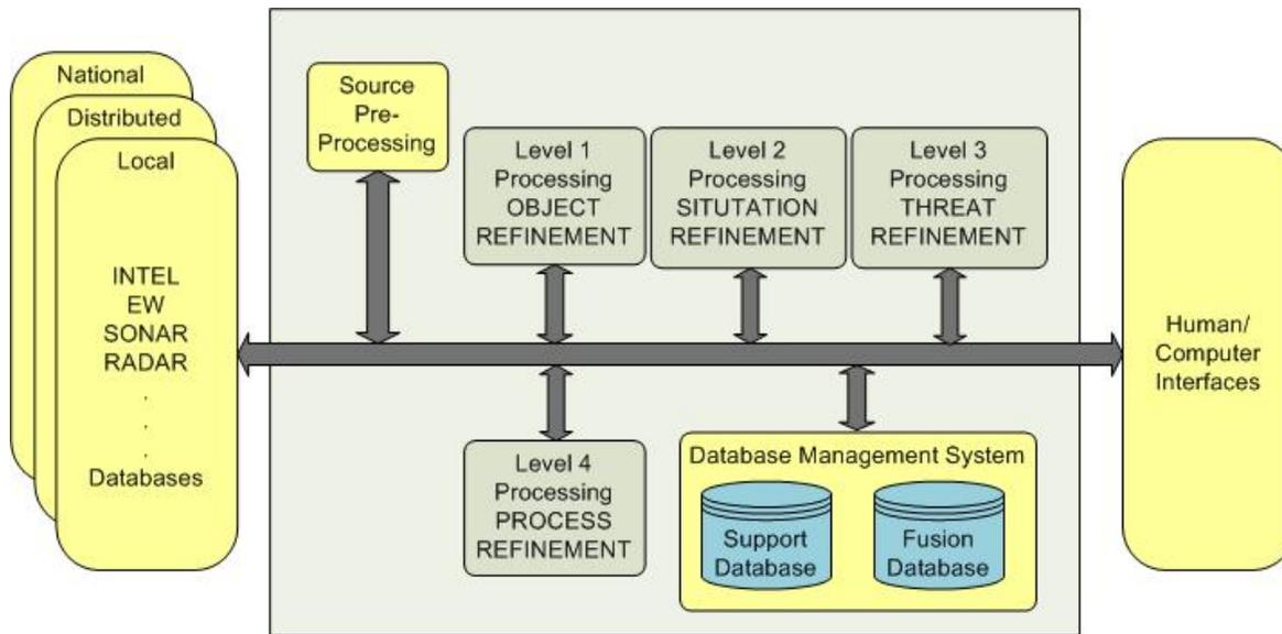
Figure 1. JDL Process Model for Data Fusion
