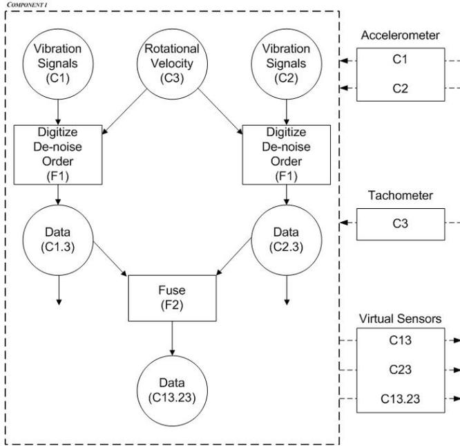
Figure 3. Intra-component fusion diagram
